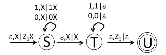
This automaton accepts strings that get to state U after consuming all of their input. Note that if it starts with an empty stack the stack will be empty at the end of the input.
