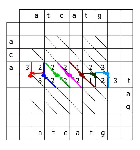
We infer that the overall cheapest path of cost 2 hits the median line at vertex (3,4):
