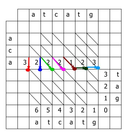
We have obtained the set of values of the best paths which run from the source till each point on the median line
